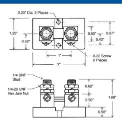
Tolerances ± .015 for the hole diameters.
