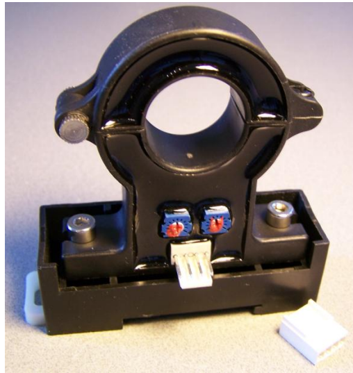
Sensor with Molex Connector (The distance between the bottom and the middle of hole is 54.8mm)
