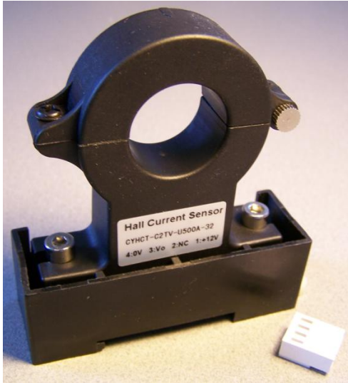
Sensor with Molex Connector (The distance between the bottom and the middle of hole is 54.8mm)
