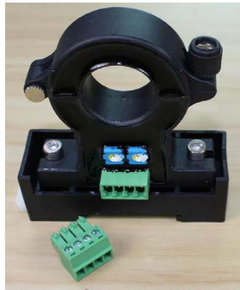
Sensor with Phoenix Connector (The distance between the bottom and the middle of hole is 54.8mm)
