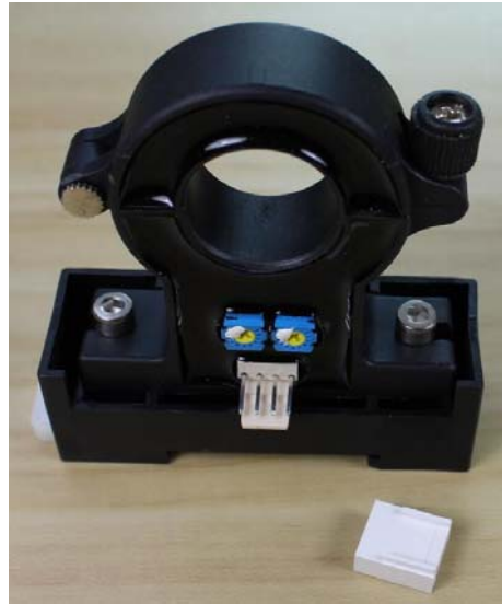
Sensor with Molex Connector (The distance between the bottom and the middle of hole is 54.8mm)
