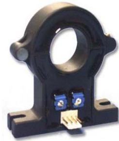
This Hall Effect current sensor is based on open loop principle and designed with a split core and a high galvanic isolation between primary and secondary circuits. It can be used for measurement of AC current, pulse currents etc. The output of the transducer reflects the real wave of the current carrying conductor.
