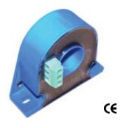
This Hall Effect current sensor is based on closed loop compensating principle and designed with a high galvanic isolation between primary and secondary circuits. It can be used for measurement of DC and AC current, pulse currents etc. The output of the transducer reflects the real wave of the current carrying conductor.
