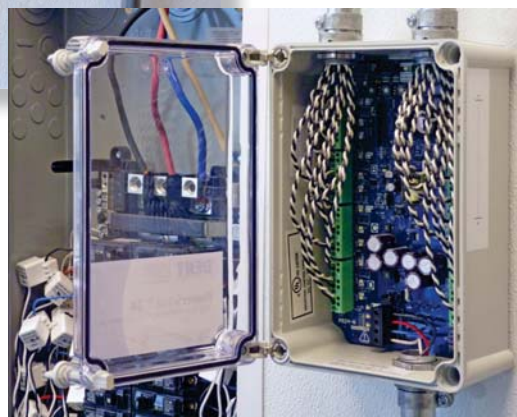
Right: The Powerscout is line-powered and the broadband power supply accommodates voltages from 80-600VAC.
