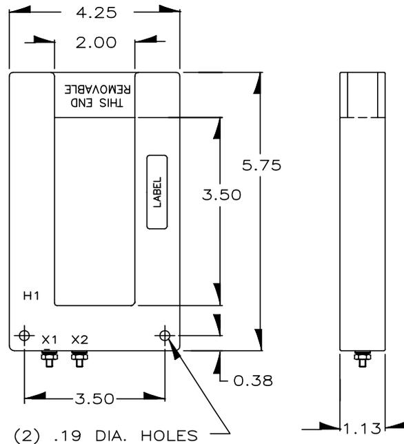
This transformer is designed for assembly to an existing electrical installation without the need for dismantling the primary bus or cables.
